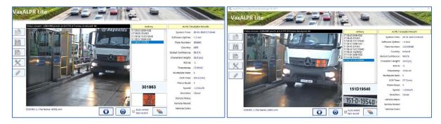
When sending the ADR plate to Helix, Vaxtor's powerful Back Office, all plate and ADR reads can be stored and subsequently searched using complex searches including part or full plates or codes. The ADR code is reported as the plate's Country Code and alarms can be triggered when an ADR plate is detected, alerting staff to any potential hazards.
