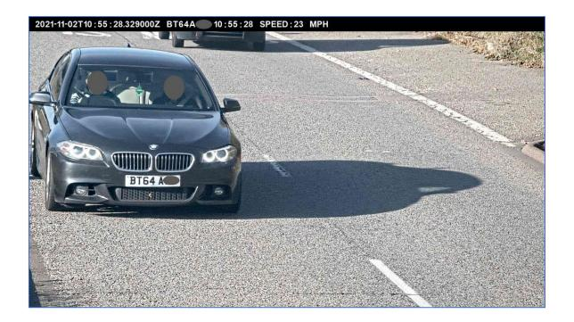
Once configured, Vax-iSpeed uses multiple image-captures to determine the speed of the vehicle as it approaches.
