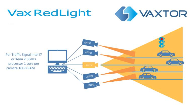
**Vax RedLight** can be configured to cover multiple lanes at intersections. Each ALPR camera views a single lane of traffic and Vax RedLight supports a maximum of 4 ALPR cameras per signal. Recognition is taken from the rear to ensure a clear image of both the traffic light and the vehicle passing through the stop line.
